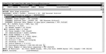
The DHCP client puts its hardware address in the DHCP discover packet because that address distinguishes that client from any other host on the network.
