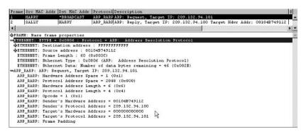
The following screen shot shows the contents of the ARP reply. The reply is a new packet and is sent from the target host. The target host is now the sender because it is sending back the requested information. In this reply packet, the source lets the destination know the source's hardware address.
