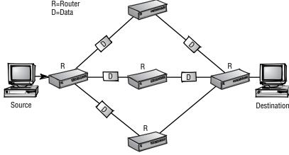
After I open the door and say, "Go," the kids enter one at a time. Entering the arcade one at a time represents the fragmenting and sending of the file. Just as each of the kids has a numbered jersey, each packet has a number so that the receiving host can put the data back together.
