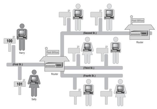
In the illustration below, the router is like a post office that routes the packets to the correct network.
