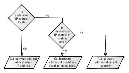
When assigning the IP address of the host, a network administrator will type in the address of the default gateway as one of the TCP/IP parameters. (The packet will be sent to the default gateway's hardware address if the packet is destined for another network.) The default gateway then determines whether the target IP address is on one of its other interfaces or whether the default gateway needs to forward the packet to another router.
