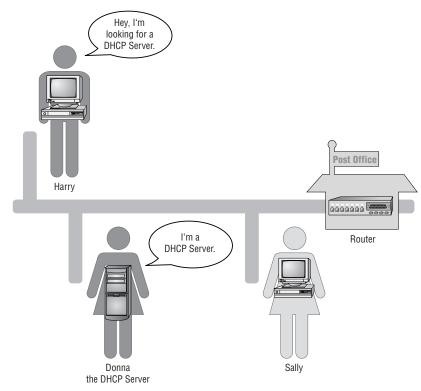
When Harry sends out the UDP packet, no connection is set up nor does Harry wait for an acknowledgment of packet receipt. Harry waits for the answer to the request, but not for an acknowledgment.
