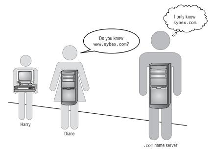
When Diane the DNS Server receives the response from the .com server, she caches the IP address of sybex.com. Diane then sends a request to the IP address of sybex.com asking for resolution to www.sybex.com.
